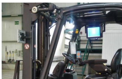
Fixed reader mounted on forklift
